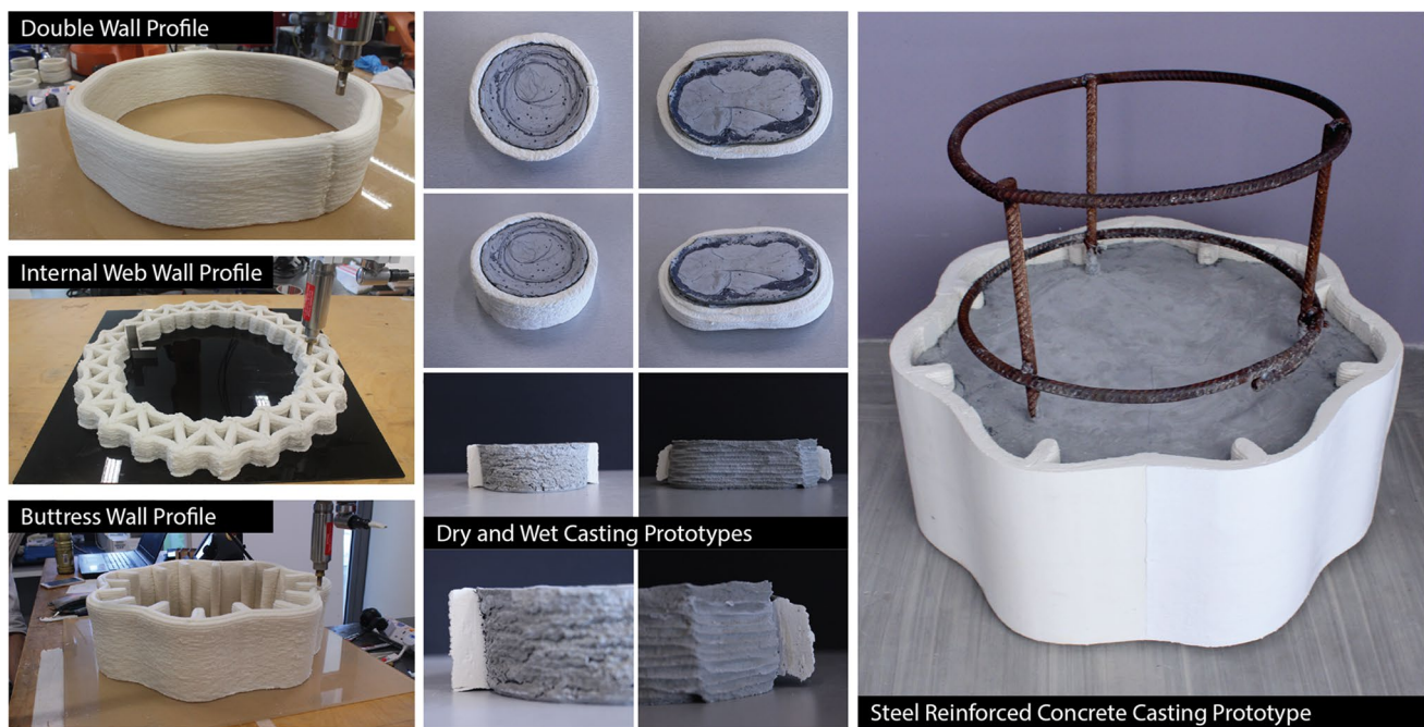
Fig. 7 Left: double, internal web, and buttress wall designs. Middle: dry cylinder and wet capsule cement casting prototypes. Cement did not penetrate the walls. Right: two buttress wall segments fused with FLAM, half sanded, half rendered, and cast with concrete
