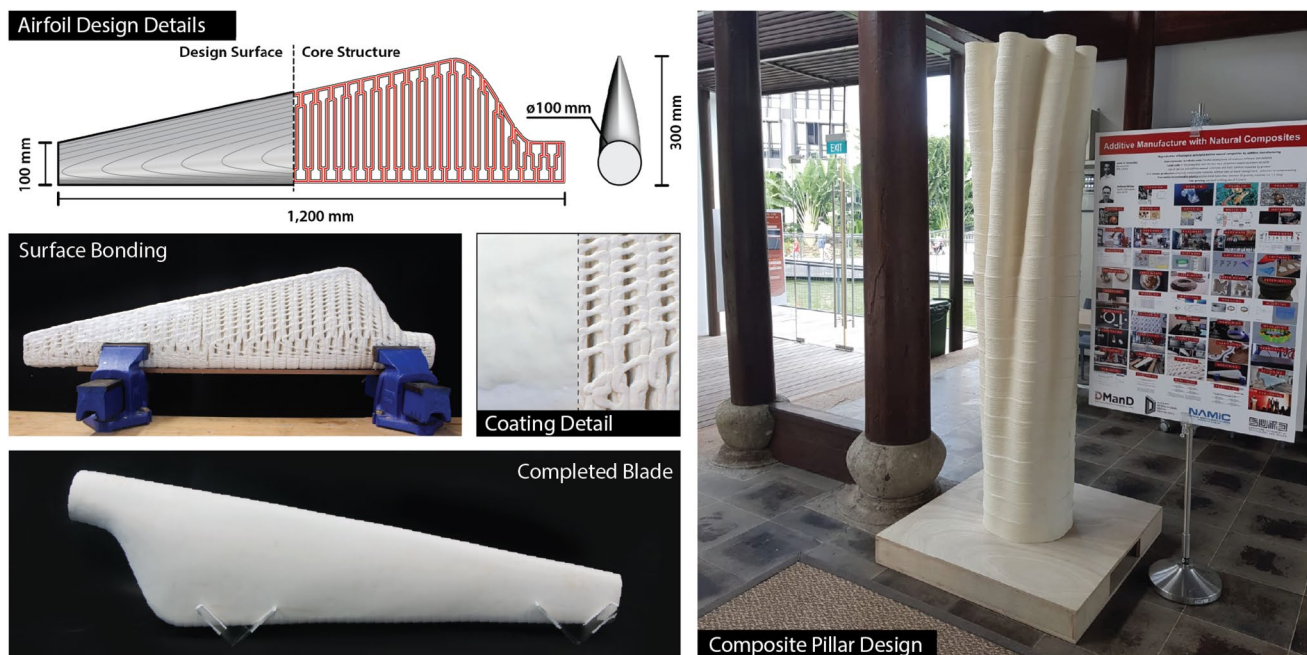
Fig. 6 Left: wind blade airfoil design evaluating hybrid fabrication combining additive manufacturing as well as conventional wood-working techniques. Right: composite pillar design work-in-progress currently 100% printed but only approximately 50% assembled
