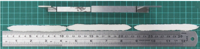
FIGURE 20. FILAMENTS PRINTED WITH FIRST SETTINGS AS OBTAINED FROM MULTI-OBJECTIVE OPTIMIZATION
